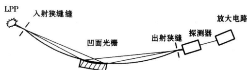
Fig. 2 Schematic diagram of setup for use in spectra measurement of LPP
