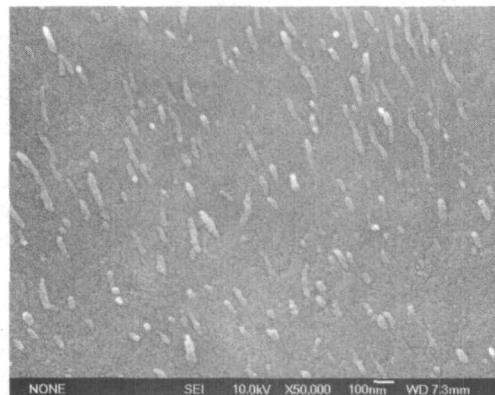
Fig. 4 SEM image of CNTs/SiO<sub>2</sub> composite gel glass
