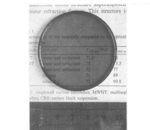
Fig 1 Photograph of CNTs / SiO<sub>2</sub> composite gel glass
