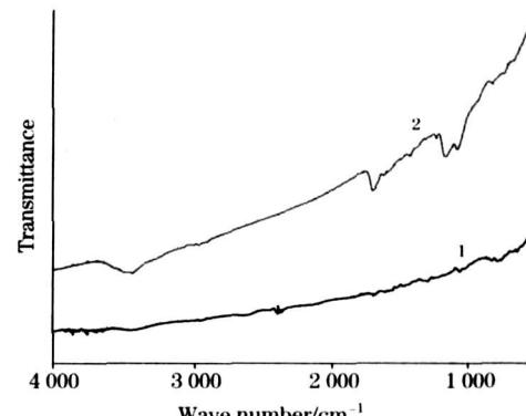
Fig 2 IR spectra of CNTs and CNTs-APTES
