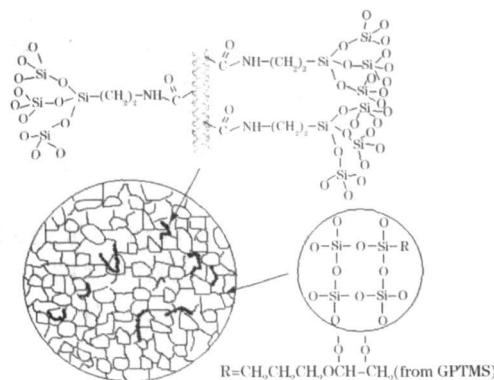
Fig. 3 Network of CNTs/SiO<sub>2</sub> composite gel glass
