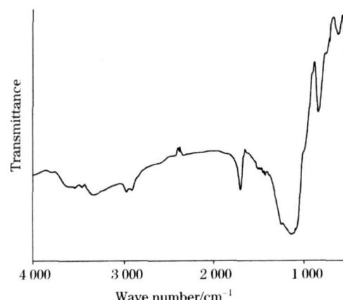
Fig. 5 IR spectra of CNTs/SiO<sub>2</sub> composite gel glass
