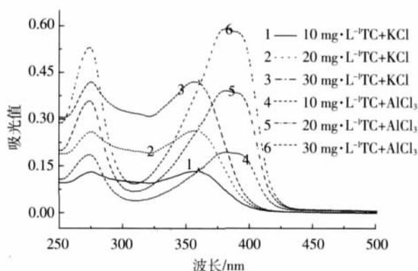
图 4 不同浓度四环素溶液中添加 Al<sup>3+</sup>前后紫外光谱图Figure 4 UV spectra of tetracycline in the presence and absence of Al<sup>3+</sup>
