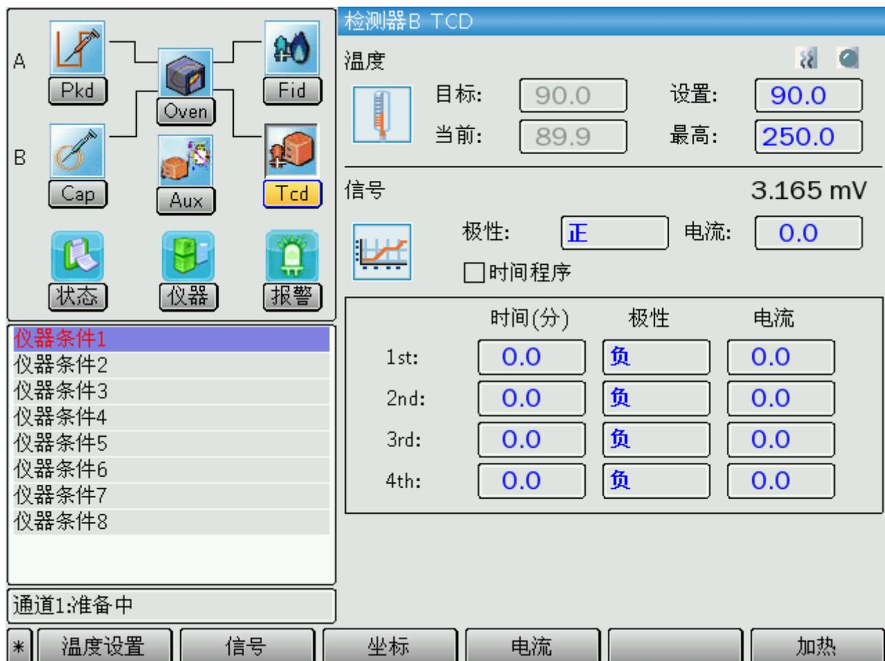
The screenshot displays the control interface for the TCD detector. It includes a main menu on the left with icons for Pkd, Oven, Fid, Cap, Aux, Tcd, 状态, 仪器, and 报警. The central panel shows the '检测器B TCD' settings, including a temperature control section with a target of 90.0, a current of 89.9, and a maximum of 250.0. The signal section shows a reading of 3.165 mV and a polarity of '正'. Below this is a table for time programs with columns for time, polarity, and current.
