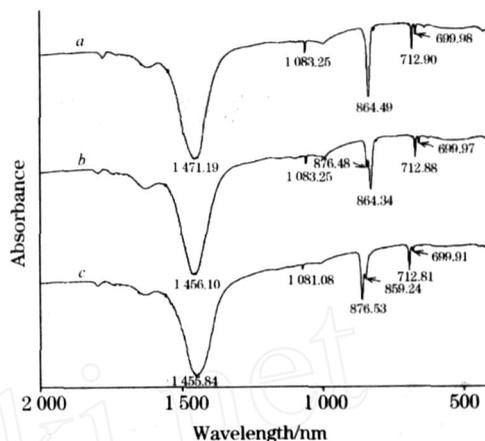
Fig 2 Typical FTIR spectra of nacre in the inner shell layers in the range of  $500 \sim 2\,000\text{ cm}^{-1}$  (a, b, c represented samples heated with 3, 6, 10 h at  $380^\circ\text{C}$  respectively)
