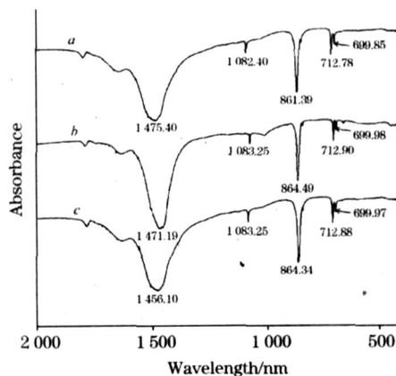
Fig 4 Typical FTIR spectra of nacre in the inner shell layers in the range of  $500 \sim 2\,000\text{ cm}^{-1}$  (a, b, c, represented samples heated 0, 3 h and 6 h at  $300^\circ\text{C}$  respectively)
