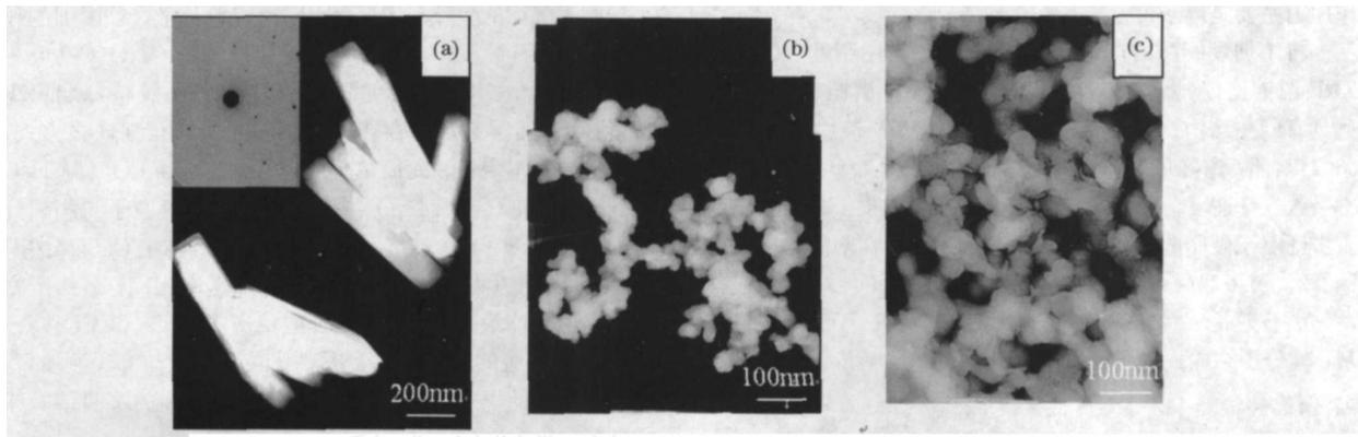
Fig 1 TEM and SAED image of the products obtained by different organic carboxylic acid
