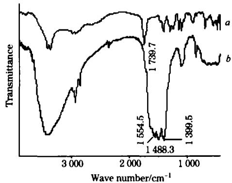
Fig 5 FTIR spectra of tartaric acid (a) and the prepared powder product (b)
