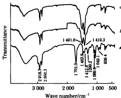
Fig 2 FTIR spectra of stearic acid and the products
