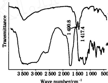
Fig 9 FTIR spectra of citric acid (a) and the product (b)
