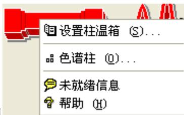
左键单击柱温箱图标，出现
