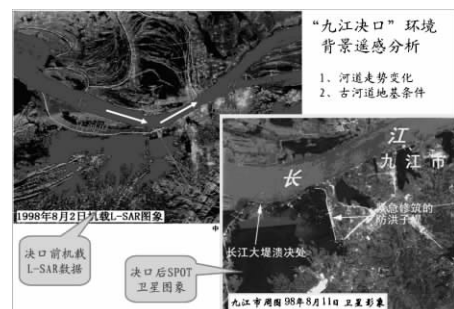
Fig 2 Analyzing the environmental background of Jiujiang dike breach based on remote sensing
