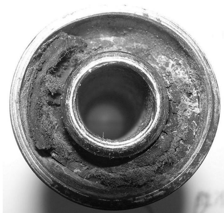
Fig 5 Broken part 2 from the brake hose
