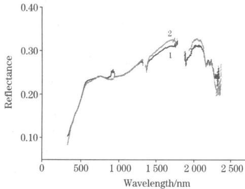
Fig. 1 Mean reflectance in Dunhuang site observed in April and July, 2002
