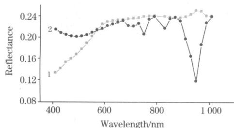
Fig. 2 CMOD IS band apparent reflectance from radiative transfer calculation in Dunhuang
