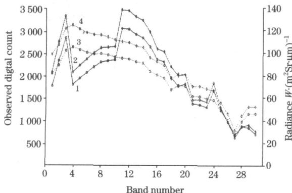
Fig. 6 DN and apparent reflectance of CMOD IS
