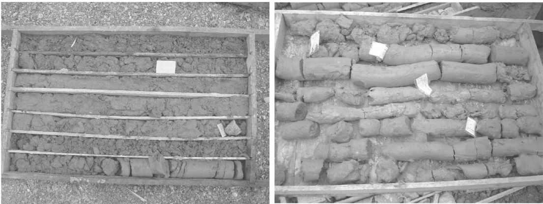
图 5 河道钻孔湖积粘土层(左: 江坪河坝址区; 右: 大野坪) Fig. 5 Lacustrine Clay of Drills(Left: Jiangpinghe Dam Area; Right: Dayeping Area)
