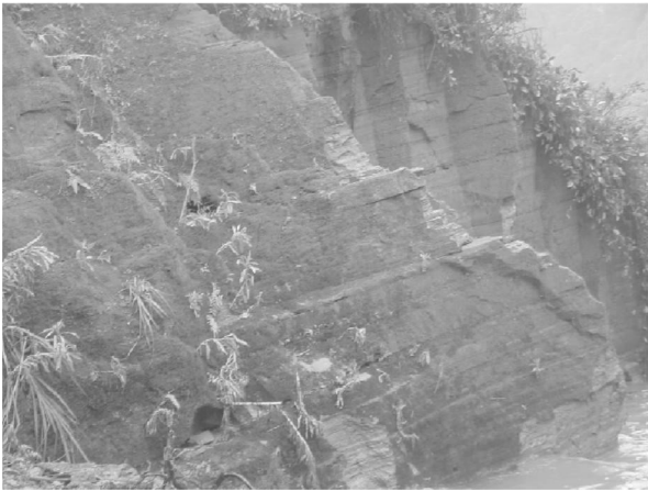
图 3 右岸 Q3 测量点沉积粘土层 Fig.3 Lacustrine Clay of Q3 Point on Right Bank
