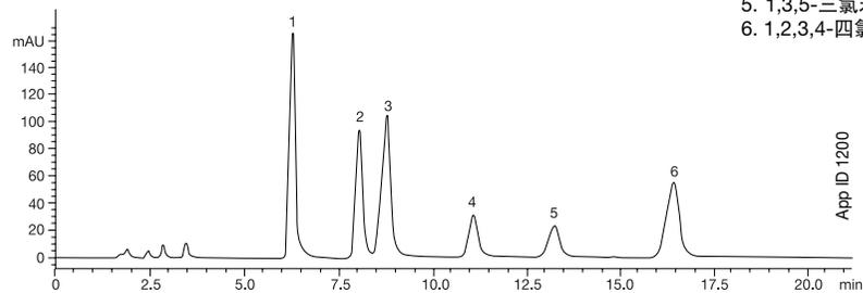
**色谱柱:** Luna 5µm Phenyl-Hexyl (苯基-己基)
