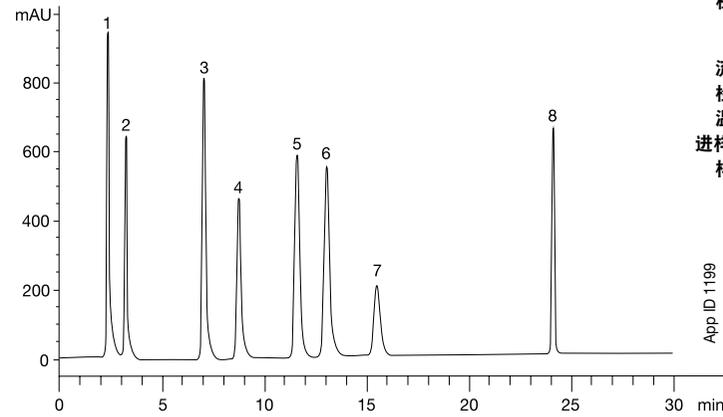
**色谱柱:** Luna 5µm Phenyl-Hexyl (苯基-己基)
