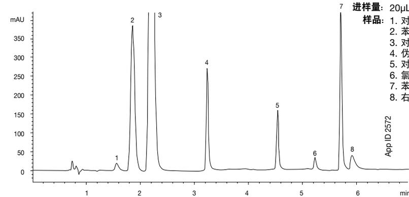
**色谱柱:** Luna 3µm Phenyl-Hexyl (苯基-己基)
