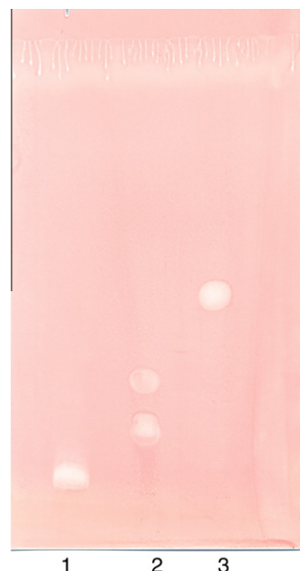
Fig. 1. TLC of Quillaja bark saponin, digitonin and shatavarin IV. Solvent system: n -butanol:water:acetic acid (84:14:7). Lane 1: saponin of Quillaja bark. Lane 2: digitonin. Lane 3: shatavarin IV. Detection: with haemolysis on the plate by immersion in erythrocytes suspension followed by washing.
