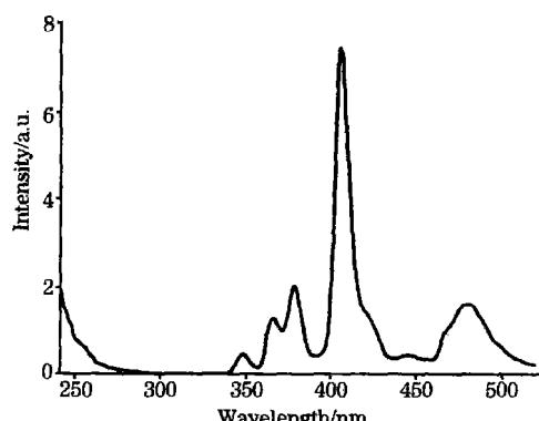
Fig. 3 Excitation spectrum of  $\text{Sm}^{3+}$  doped BLBL glasses
