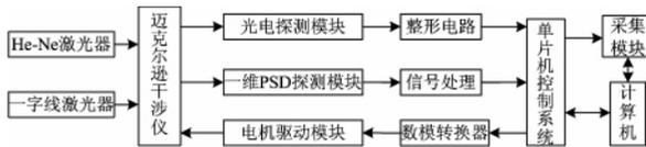
Fig 2 The control and sampling system of spectrometer
